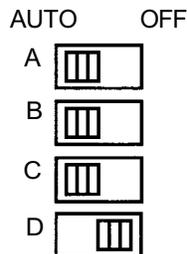
Set the front-mounted AUTO/OFF switches of A, B, and C channels to AUTO and that of D channel to OFF.
