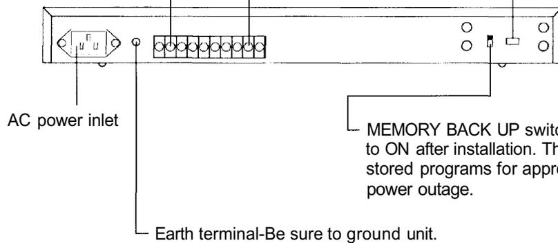
**MEMORY BACK UP switch**-Be sure to set this switch to ON after installation. This switch protects clock and stored programs for approximately 100 hours during power outage.
