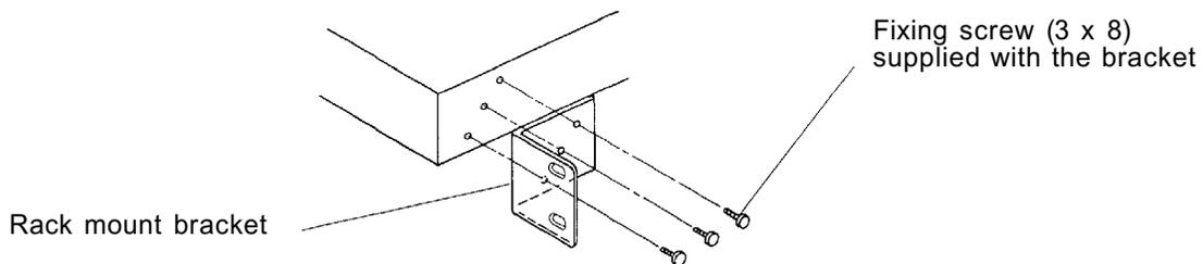
2. Fix the TT-104B in the rack using screws supplied with the bracket. See the figure.
