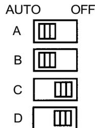
2) To operate the shorter school hour program, set the AUTO/OFF switch of the C channel to AUTO, while setting it to OFF for all the other channels.
