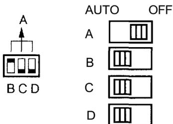
If the CHANNEL ASSIGNMENT switch of B channel is set to ON and the AUTO/OFF switch of A channel to OFF in Example 1.
